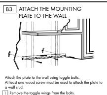
1 Insert the bolts into the mounting plate through the holes designated to go into drywall and reattach the toggle wings 3/4" onto each bolt.
